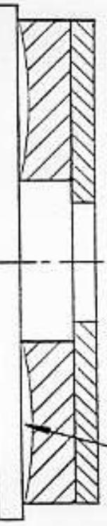
CORRECTION: TO CORRECT THIS CONDITION MOVE ONE CONDITIONING RING OUT AND ONE IN. MOVE THE OTHER CONDITIONING RING(S) IN AND OUT IF DISHING IS EXCESSIVE.
