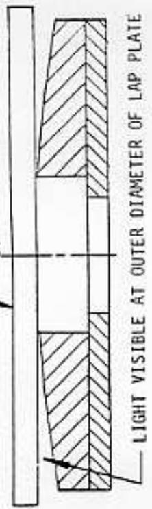
CORRECTION: TO CORRECT THIS CONDITION, MOVE ONE OF THE CONDITIONING RINGS INWARD TOWARD THE CENTER. MORE THAN ONE RING SHOULD BE MOVED IF WEAR IS EXCESSIVE.
